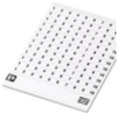
Marker card, Card, white, labeled, horizontal: consecutive numbers 1 ... 10, 11 ... 20, etc. up to 91 ... (99)100, mounting type: adhesive, for terminal block width: 6.2 mm, lettering field size: 6.2 x 3.8 mm
