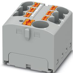
Distribution block, nom. voltage: 450 V, nominal current: 41 A, connection method: Push-in connection, Push-in connection, number of connections: 7, cross section: 0.2 mm<sup>2</sup> - 6 mm<sup>2</sup>, AWG: 24 - 10, width: 27.9 mm, height: 21.7 mm, color: gray, mounting type: for snapping onto a DIN rail adapter, Direct mounting with flange, Free-hanging
